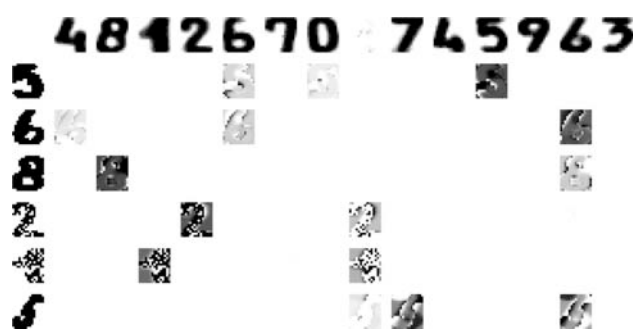
Fig. 10 Results on artificially corrupted binary handwritten digit images where some pixels have been turned to white. The images on the top line depict the reshaped parameters a_{tk} as basis images. Some examples from this data set are shown in the first column, and their analysis as provided by the AB model in the next columns. For each datum instance n and each aspect k , the probability values q_{k,t,n,x_m} are shown for each pixel t \in \{1, \dots, 240\} . On all these plots, the level of darkness of a pixel is proportional to the probability of it being ‘on’
