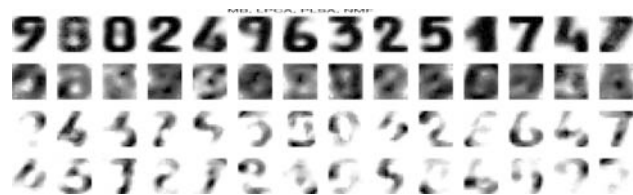
Fig. 11 Basis images estimated by MB ( top row ), LPCA ( second row ), PLSA ( third row ) and NMF ( bottom row ) in artificially corrupted binary handwritten digits
